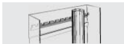
Rack for cables in vertical zone
